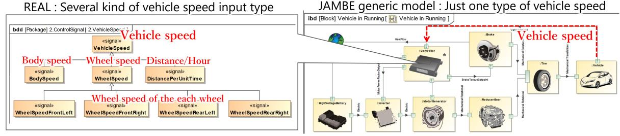
The controller behavior cannot be reproduced without correct inputs. →It needs to create a wrapper model for all controller inputs.
