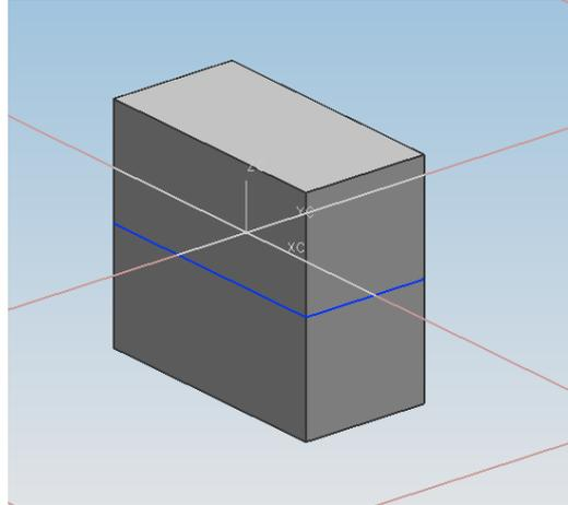
Figure 7-7: Symmetric Extrusions
