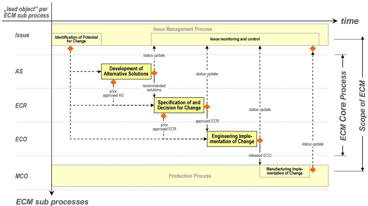
**Figure 4: Simplified overall picture of the dependencies of the phases of the SASIG ECM Reference Process**
